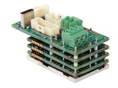
The **FXM060-5-EM** is an Extended Environment single-axis servo drive and integration board assembly for a FXE060-5-EM FlexPro® series servo drive with IMPACT<sup>TM</sup> architecture. Connections to the controller, motor, power, and feedback are simplified through the standard connectors featured on the board.
