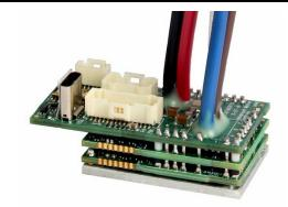
The **FXM060-25-CM** is an Extended Environment single-axis servo drive and integration board assembly for a FXE060-25-CM FlexPro® series servo drive with IMPACT<sup>TM</sup> architecture. Connections to the controller, motor, power, and feedback are simplified through the standard connectors featured on the board.
