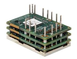
The **FXE060-10-EM** is a FlexPro® series Extended Environment servo drive with IMPACT<sup>TM</sup> architecture.
