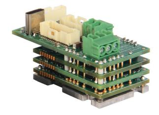
The **FM060-5-EM** is a single-axis servo drive and integration board assembly for a FE060-5-EM FlexPro® series servo drive with IMPACT<sup>TM</sup> architecture. Connections to the controller, motor, power, and feedback are simplified through the standard connectors featured on the board.
