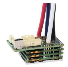
The **FM060-45C-EM** is a single-axis servo drive and integration board assembly for a FE060-45C-EM FlexPro® series servo drive with IMPACT<sup>TM</sup> architecture. Connections to the controller, motor, power, and feedback are simplified through the standard connectors featured on the board.
