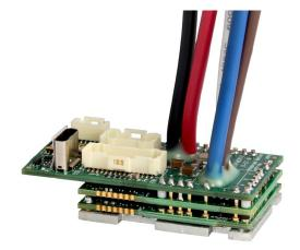
The **FM060-25-CM** is a single-axis servo drive and integration board assembly for a FE060-25-CM FlexPro® series servo drive with IMPACT<sup>TM</sup> architecture. Connections to the controller, motor, power, and feedback are simplified through the standard connectors featured on the board.
