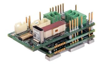
The **FM060-10-RM** is a single-axis servo drive and integration board assembly for a FE060-10-RM FlexPro® series servo drive with IMPACT<sup>TM</sup> architecture. Connections to the controller, motor, power, and feedback are simplified through the standard connectors featured on the board.
