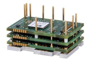
The **FE060-5-EM** is a FlexPro<sup>®</sup> series servo drive with IMPACT<sup>TM</sup> architecture.
