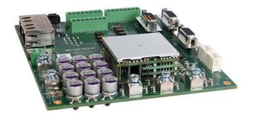
The **FD100-50-CM** is a servo drive and development board assembly for a FE100-50-CM FlexPro<sup>®</sup> series servo drive with IMPACT<sup>TM</sup> architecture. Connections to the controller, motor, power, and feedback are simplified through the standard connectors featured on the board. The **FD100-50-CM** is ideal for prototyping and can be used in production and industrial environments as well.
