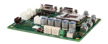
The **FD060-5-RM** is a servo drive and development board assembly for a FE060-5-RM FlexPro<sup>®</sup> series servo drive with IMPACT<sup>TM</sup> architecture. Connections to the controller, motor, power, and feedback are simplified through the standard connectors featured on the board. The **FD060-5-RM** is ideal for prototyping and can be used in production and industrial environments as well.
