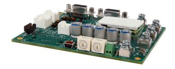
The **FD060-45C-CM** is a servo drive and development board assembly for a FE060-45C-CM FlexPro<sup>®</sup> series servo drive with IMPACT<sup>TM</sup> architecture. Connections to the controller, motor, power, and feedback are simplified through the standard connectors featured on the board. The **FD060-45C-CM** is ideal for prototyping and can be used in production and industrial environments as well.
