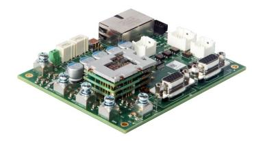
The **FD060-25-EM** is a servo drive and development board assembly for a FE060-25-EM FlexPro<sup>®</sup> series servo drive with IMPACT<sup>TM</sup> architecture. Connections to the controller, motor, power, and feedback are simplified through the standard connectors featured on the board. The **FD060-25-EM** is ideal for prototyping and can be used in production and industrial environments as well.
