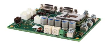
The **FD060-25-CM** is a servo drive and development board assembly for a FE060-25-CM FlexPro<sup>®</sup> series servo drive with IMPACT<sup>TM</sup> architecture. Connections to the controller, motor, power, and feedback are simplified through the standard connectors featured on the board. The **FD060-25-CM** is ideal for prototyping and can be used in production and industrial environments as well.
