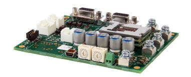
The **FD060-10-CM** is a servo drive and development board assembly for a FE060-10-CM FlexPro<sup>®</sup> series servo drive with IMPACT<sup>TM</sup> architecture. Connections to the controller, motor, power, and feedback are simplified through the standard connectors featured on the board. The **FD060-10-CM** is ideal for prototyping and can be used in production and industrial environments as well.
