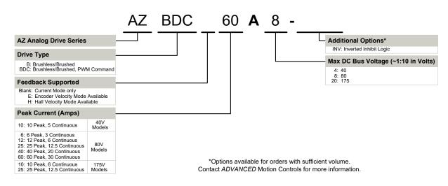
ADVANCED Motion Controls AZ series of servo drives are available in many configurations. Note that not all possible part number combinations are offered as standard drives. All models listed in the selection tables of the website are readily available, standard product offerings.
