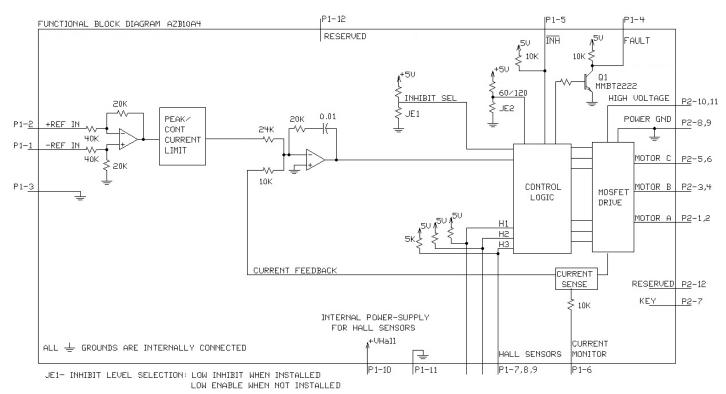
JE2- PHASING: 120 DEGREE WHEN INSTALLED, 60 DEGREE WHEN NOT INSTALLED
