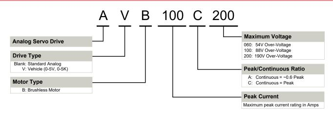
ADVANCED Motion Controls servo drives are available in many configurations. Note that not all possible part number combinations are offered as standard drives. All models listed in the selection tables of the website are readily available, standard product offerings.
