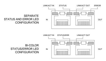
LINK/ACT IN and LINK/ACT OUT are used to drive the corresponding LINK IN and LINK OUT LEDs on a typical RJ-45 connector. The two STATUS/ERR pins are used to drive a bi-color Status LED or two separate single-color LEDs, depending on the user
