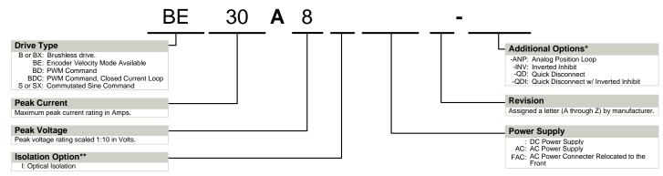
ADVANCED Motion Controls analog series of servo drives are available in many configurations. Note that not all possible part number combinations are offered as standard drives. All models listed in the selection tables of the website are readily available, standard product offerings.
