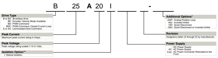
\* Options available for orders with sufficient volume. Contact ADVANCED Motion Controls for more information. \*\* Isolation comes standard on all AC supply drives and most DC supply drives 200V and above. Consult selection tables of the website or the drive datasheet block diagram to see if isolation is included.
