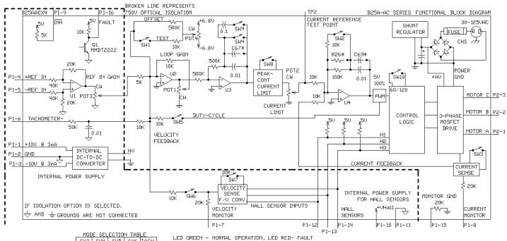
RECOMMENDED SETTING FOR CURRENT MODE — POTI FULLY CCW, POT3 FULLY CW
